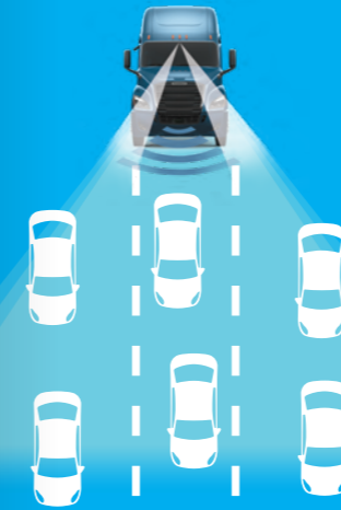
Detroit Assurance radar reports the distance, velocity, width, lateral offset, type, and confidence level of the top six priority vehicles in the truck's path.
